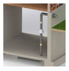
Many municipalities are being proactive in requiring a full vent stack to reduce radon levels in homes and have dedicated radon programs for new construction. As a minimum, it is critical to install the sub-slab pipe and radon rough-in stub (Level-1) as per the National Building Code 2015 requirements in the event that future radon mitigation is required.
