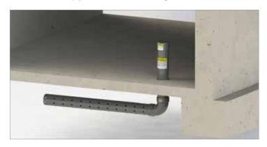
The capped rough-in stub (Level-1) is not a complete radon reduction system. It only allows the future addition of a full passive or active piping system if the home tests high for radon after occupancy.
