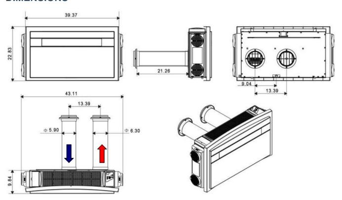
**Note:** The external pipes have two different diameters, use  $\emptyset$ 6.30 in for air outlet side ( see red arrow ) and  $\emptyset$ 5.90 in for air inlet side ( see blue arrow ).
