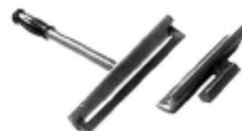
CLEATER Ideal tool to attach cleat to Ductmate 25/35 Flange Joint where space is not a consideration. Use Cleater II in conjunction with 5/8" deep-wall socket, extensions and wrench (not included) to attach cleat to Ductmate 25/35 in hard to reach places.
