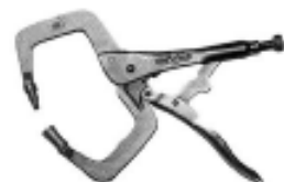
CORNER ALIGNMENT TOOL Modified vice grip can facilitate installation of corner clips.
