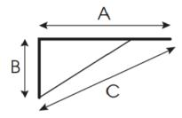
ACB-30: (A)30" (B)16" (C)34" ACB-36: (A)36" (B)16" (C)39" ACB-42: (A)42" (B)16" (C)43" ACB-48: (A)48" (B)16" (C)51"
