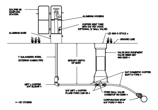
Sampling Stations shall be 'bury, with a 3/4" FIP inlet, and a (3/4" hose or unthreaded) nozzle.
